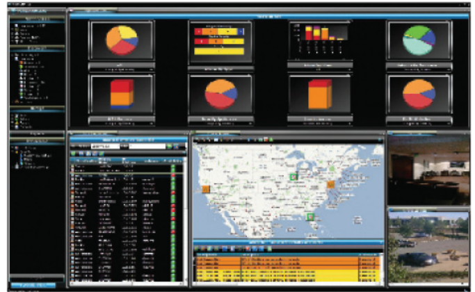
▲ NeuralStar integrates all network event data—availability, performance, security, and more from any network connected port, device, service or application - all on a single console.
