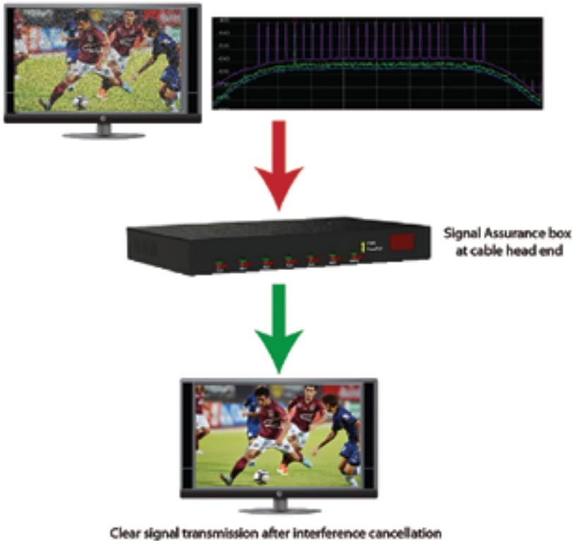
*In Kratos' model, the interfering signal is characterized to create an inverted copy of the interferer using firmware. The inverted signal is then fed into the interfering signal, thereby cancelling it.*
