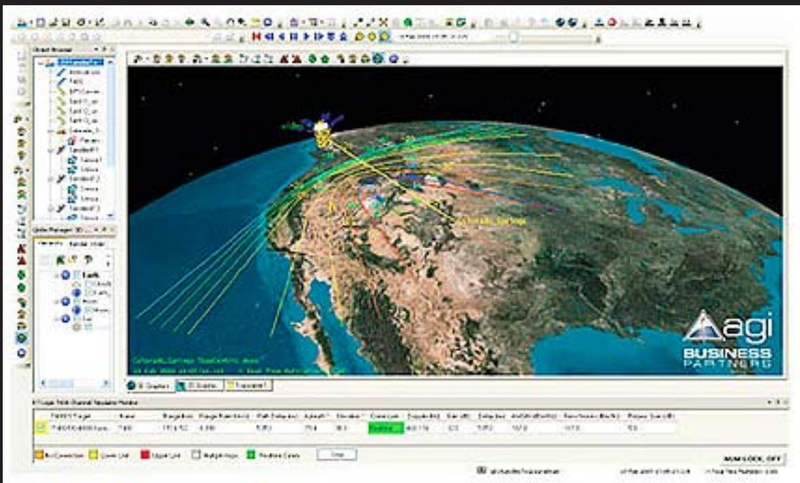
Often employing multiple remote sensors, today's interference detection systems combine signal data from geographically dispersed fixed and moving locations for enhanced overall situational awareness. Further development of such systems is proceeding rapidly, with key focus on faster detection of a broader range of interference types in wider frequency segments. Reductions in system size, complexity
